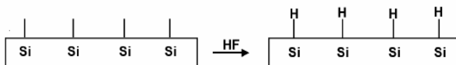
Fig.9a Hydrogenation of silicon surface
